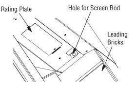
Figure 35 - Installing Fireplace Screen
