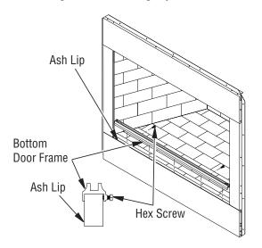
Figure 40 - Installing Bottom Door Frame
