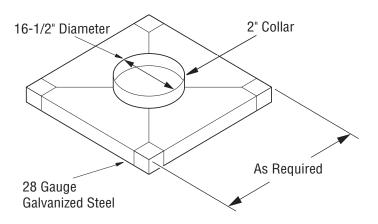
Figure 26 - Constructing Chase Top Flashing
