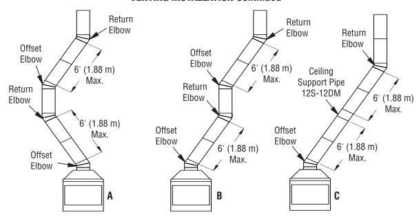
Figure 12 - Typical Offset Terminations
