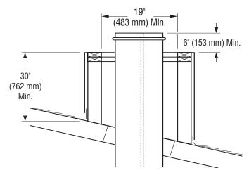
Figure 25 - Constructing Chase
