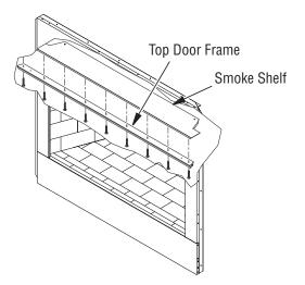
Figure 39 - Installing Top Door Frame
