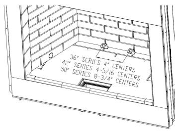
Figure 36 - Installing Grate Retainers
