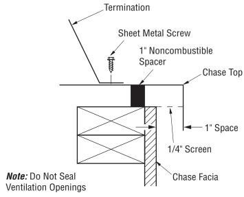
Figure 24 - Securing Termination to Chase Top Flashing with Sheet Metal Screws
