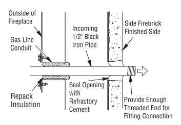
Figure 38 - Gas Line Installation
