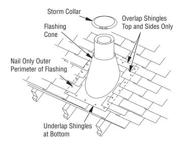
Figure 16 - Flashing Installation
