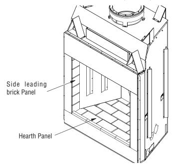
Figure 31 - Installing Hearth and Leading Brick panels
