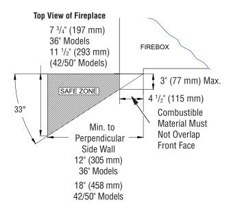
Figure 7 - Mantel Clearances to Combustible Material
