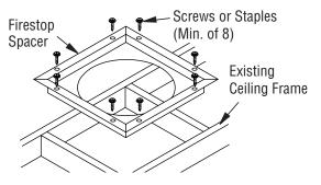
Figure 14 - Firestop Spacer with Attic Space Above Ceiling
