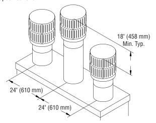
Figure 19 - Multiple Chase Installation
