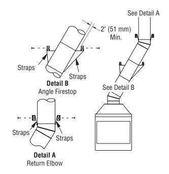
Figure 11 - Ceiling Support Pipe 12S-12DM
