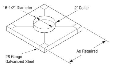
Figure 22 - Constructing Chase Top Flashing
