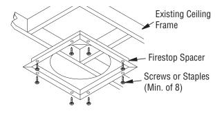
Figure 13 - Firestop Spacer with Living Space Above Ceiling
