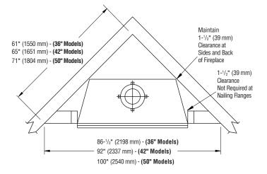
Figure 5 - Corner Installation
