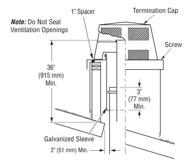
Figure 23 - Installing Termination Cap
