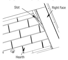
Figure 32 - Slots for Firebrick Walls
