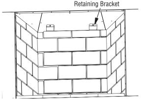
Figure 34 - Installing Rear Wall
