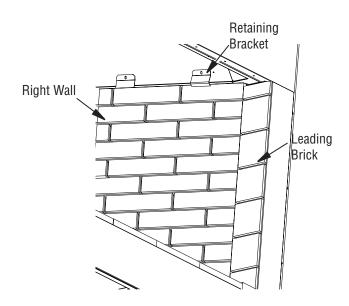
Figure 33 - Installing Side Walls
