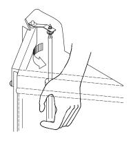
Figure 42 - Adjusting Bi-Fold Doors
