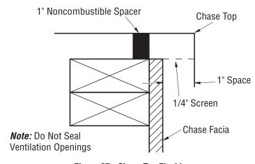
Figure 27 - Chase Top Flashing
