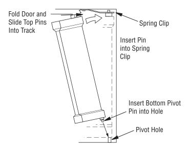
Figure 41 - Installing Bi-Fold Doors
