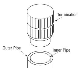
Figure 28- Installing Termination Cap
