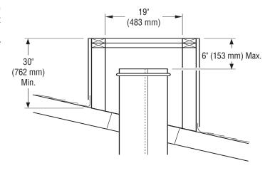
Figure 21 - Constructing Chase
