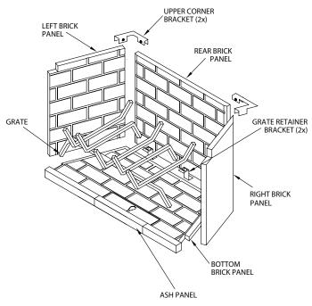
Figure 36a - Installing Refractory Panels
