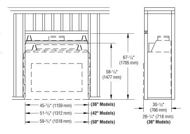
Figure 4 - Framing Dimensions
